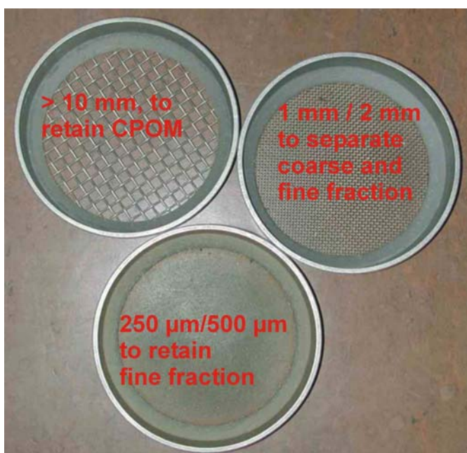
FIGURE 8.1: Set of sieves to be used for separating the coarse and the fine fraction.
