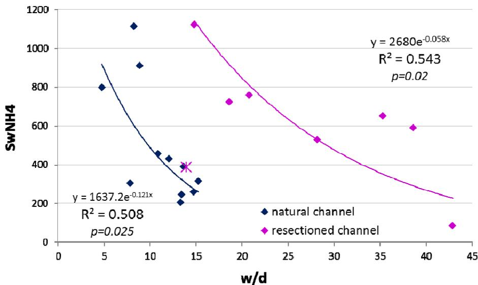
Fig. 7 – Relationship between the width and depth channel ratio ( $w/d$ ) and the  $NH_4$  uptake length ( $Sw_{NH_4}$ ) in the Sardinian sites.
