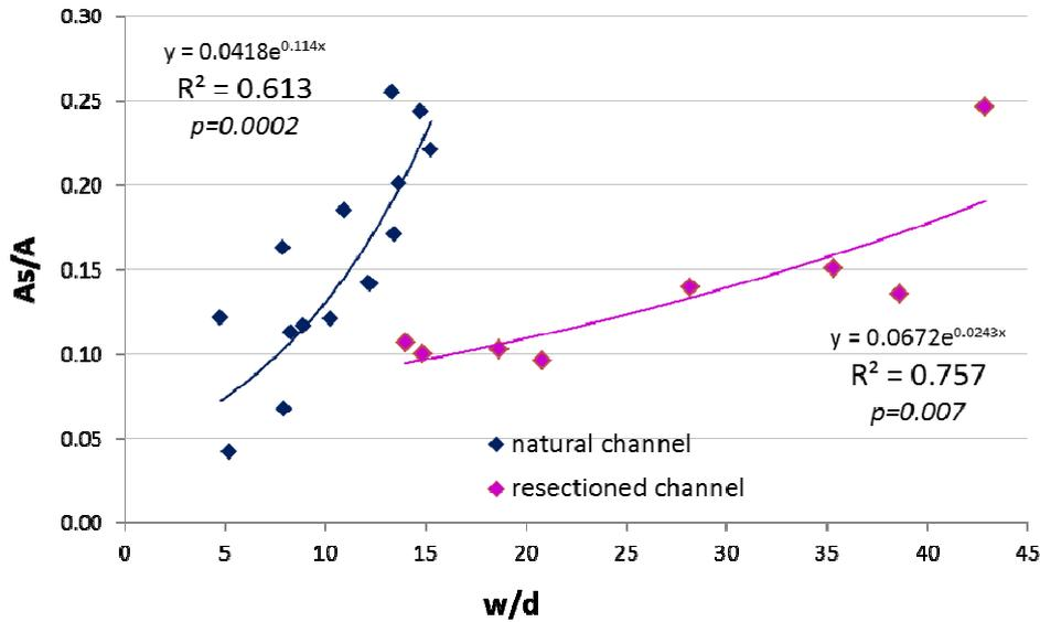
Fig 4 – Relationship between the width and depth channel ratio (w/d) and the normalized storage area (As/A) in the Sardinian sites.
