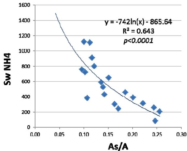
Fig. 13. Relationship between transient storage area ( $As/A$ ) and the uptake length of  $NH_4$  for the Sardinian river stretches examined.
